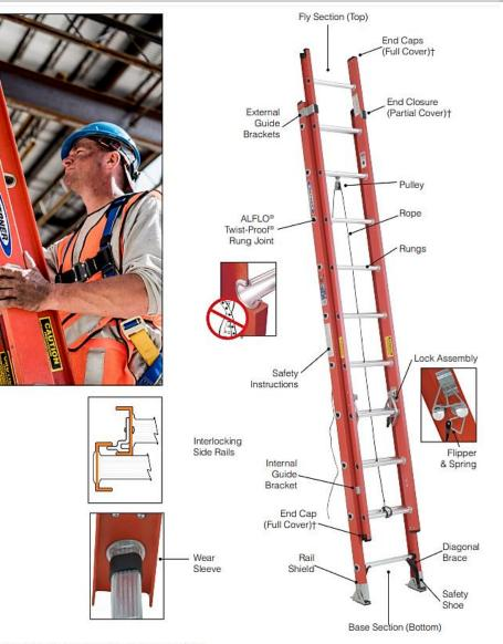
† End Cap's and End Closure's positions differ by ladder models. End Caps - completely cover the rail. End Closures - partially cover the rail, leaving clearance for the mating ladder section.
